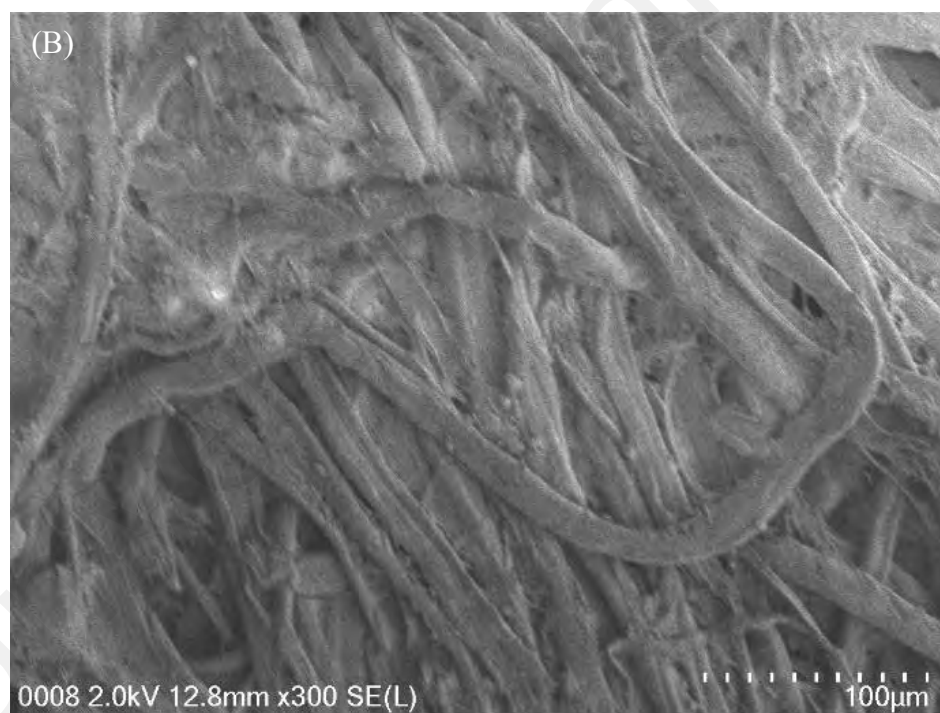
Figure 4.35: FESEM images of blank filter paper before combustion with paddy straw
