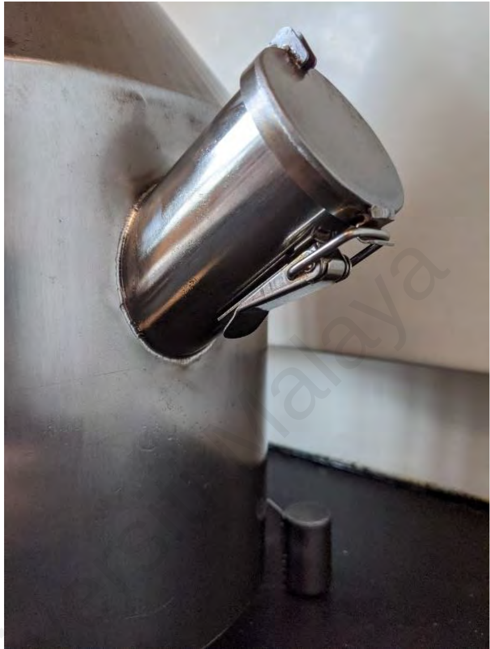
Figure 3.8: The opening of the muffler that was tightly secured to ensure no smoke escaped during combustion
