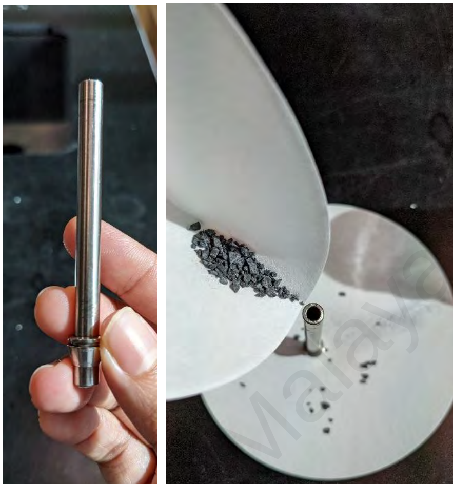
Figure 3.6: AC holder (left). AC inserted into AC holder (right)
