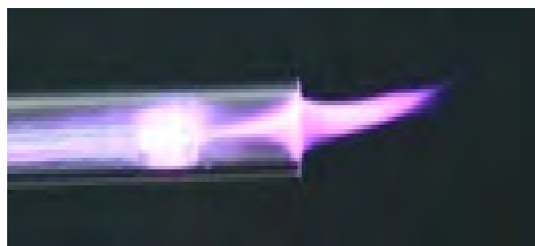
Figure 2.1: Spark of plasma generated from plasma jet device (adapted from Joh et al. , 2014).
