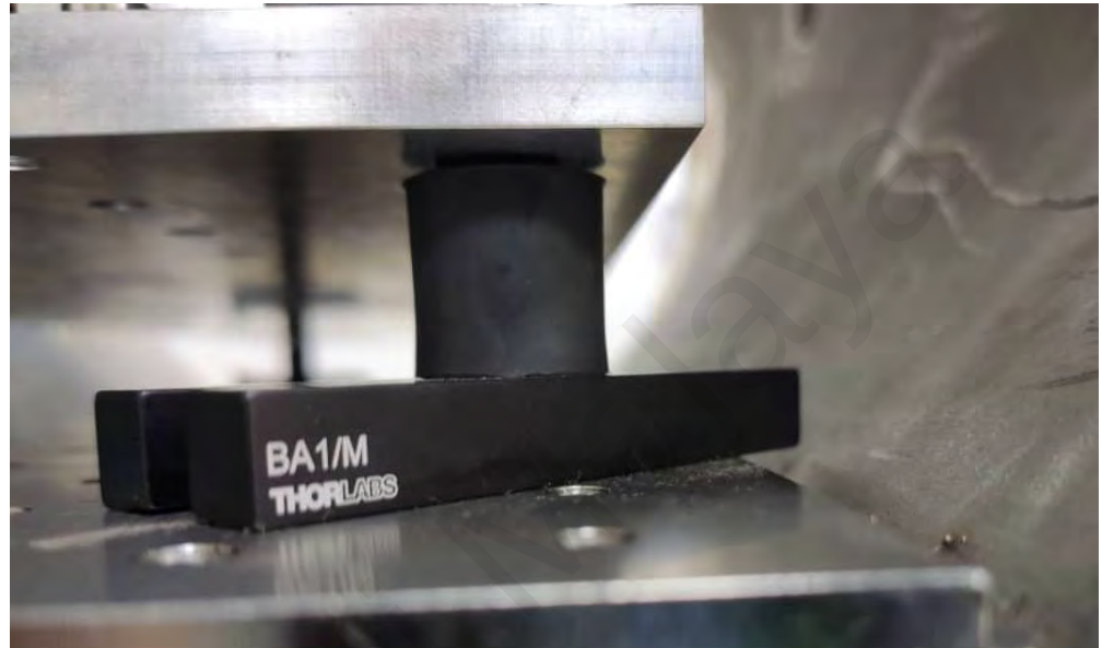
Figure 3.15: Anti-vibration mounts for the base plate.
