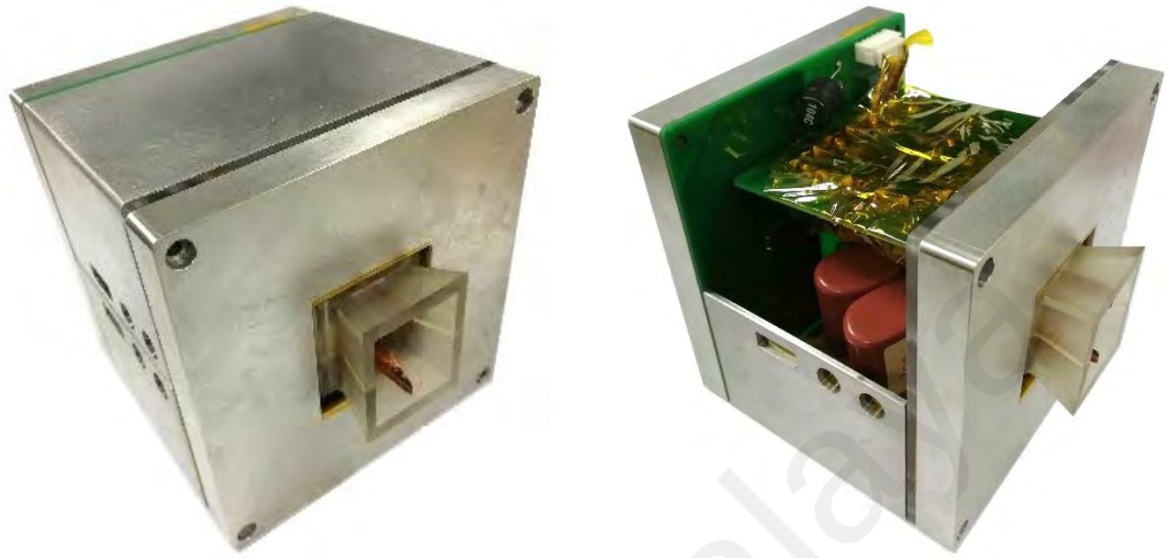
Figure 3.3: Exterior and interior views of the PPT unit.
