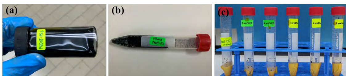
Figure 3.3: Illustration of (a) Pristine PEDOT:PSS solution, (b) Filtered by 0.45 \mu\text{m} filter and (c) Added with different amount of EG
