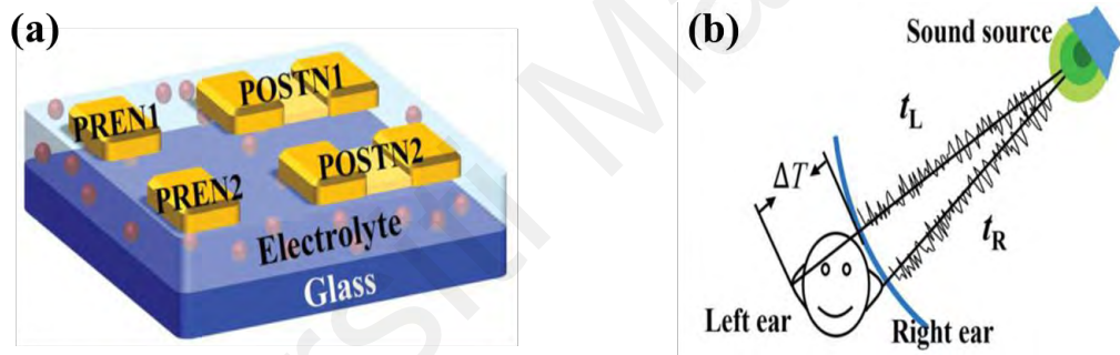
Figure 2.16: Schematics of (a) Sound location using a neuro-transistor-based artificial neural network, (b) Sound location by the human brain binaural effect (Wan et al., 2018)
