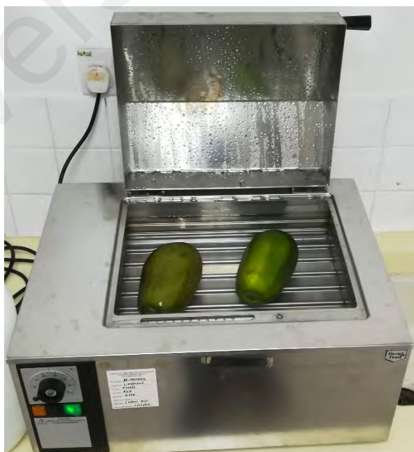
Figure 3.4: Hot water treatment of papaya in a water bath at 54 °C for 5 min.
