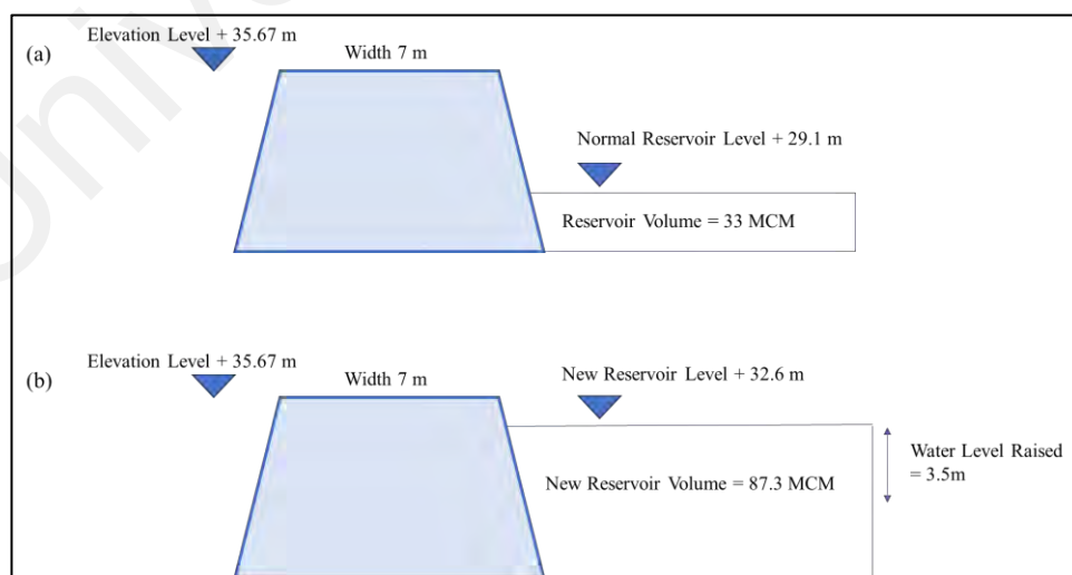
Figure 3.13: New Standard feature for the Timah Tasoh Dam (under construction); a) Current feature and b) Future feature (Ismail, 2012).
