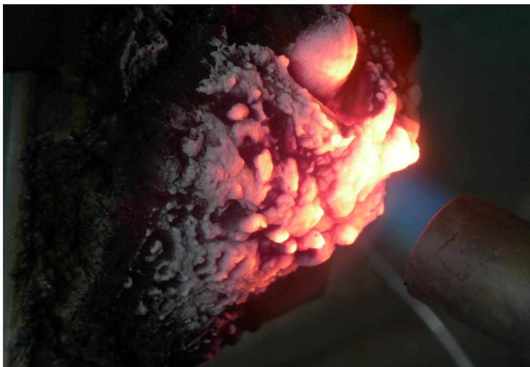
Figure 4.14 The steel plate coated with C3 formulation during fire test
