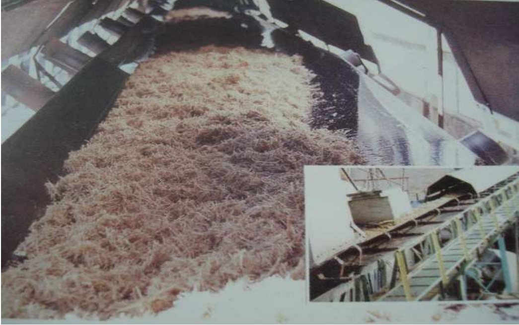
Figure 4.3: Transported the Bagasse through the conveyer belts from the sugarcane factory to the paper factory
