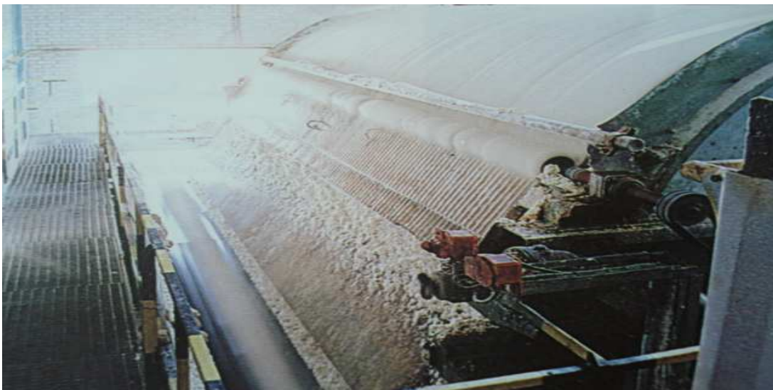
Figure 4.5 : Pulp Screening and Cleaning in Pars Paper Factory
