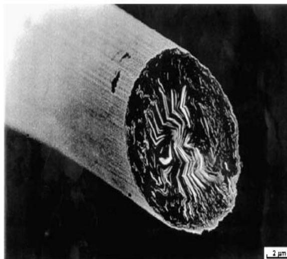
Figure 2.2: Micrograph of a mesocarbon fiber (MCF) [Takamura, 2002].
