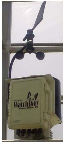
Figure 3.11: Wind speed and wind direction sensor.
