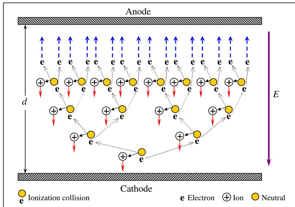
**Figure 2.2 :** Townsend Breakdown Mechanism.
