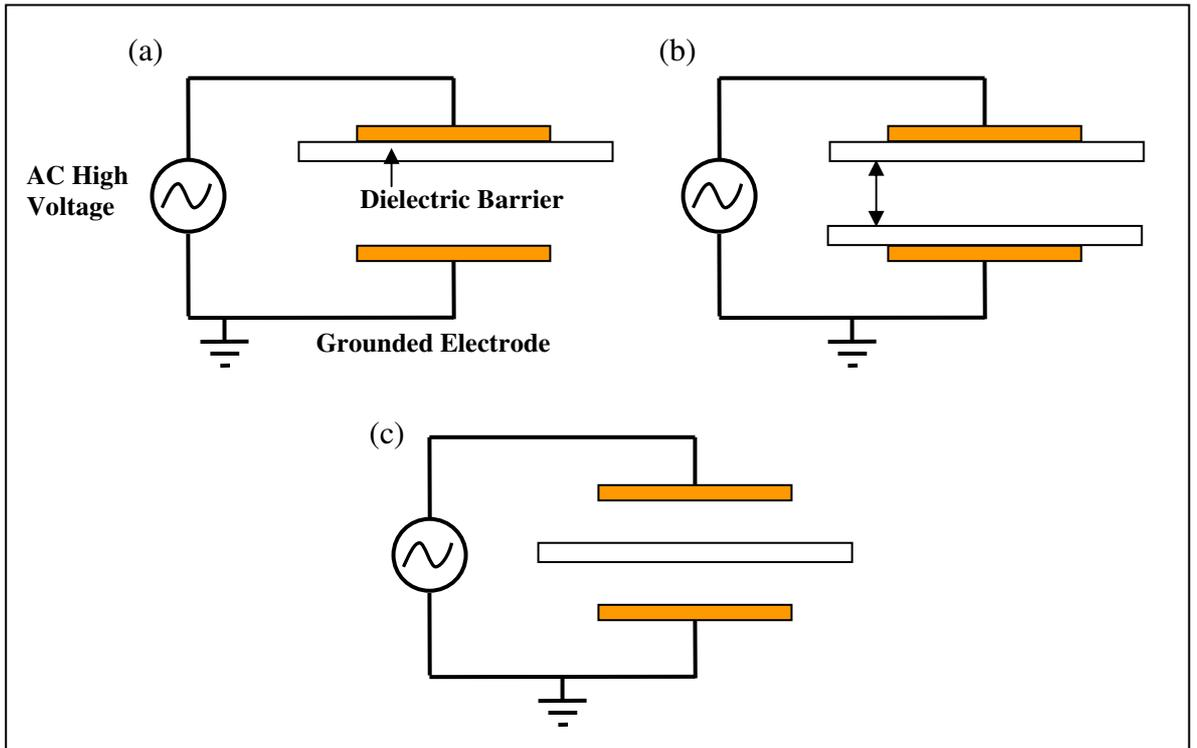
**Figure 2.1** : Various parallel plate electrodes configuration of DBD with the dielectric barrier layer(s) at different positions as shown.
