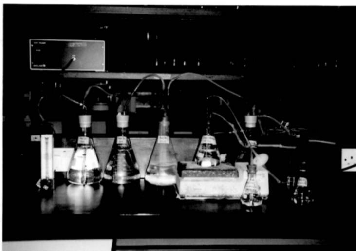
**Figure A-2: A typical set up of Sturm-test for Run 3. (The apparatus was reset up after the actual experiment has completed. Only one reactor is shown. The volume of CO<sub>2</sub> scrubber was not the actual volume used in the experiment).**
