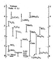
Figure 1.1: The range of intercalation potentials for various materials (Guyomard and Tarascon, 1994).
