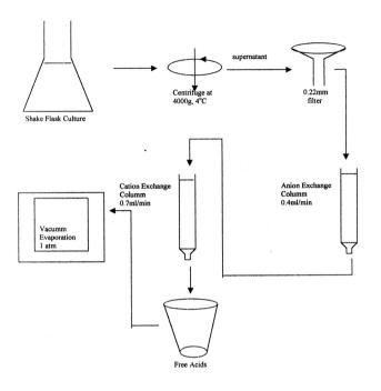
Figure 3.1: Shows the schematic diagram of the process of recovery and purification of lactic acid from the fermentation broth
