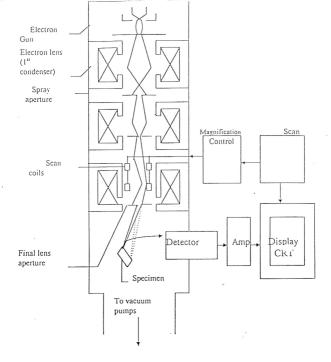
Figure 11 : Schematic drawing showing the electron column, the deflection system and the electron detectors
