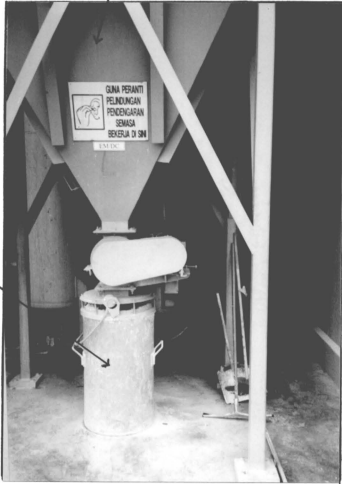
Plate 3 Barrel collecting Water-Based Paint Dust from Hopper
