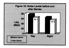
Levels of noise was found to be approximately 10 dB lower after the barrier compared to before the barrier. Day time noise levels after the barrier was 64.1,66.0 and 65.1 dB(A) over three samplings. The night time noise levels after the barrier was 55.8.55.4 and 55.3 dB(A).
