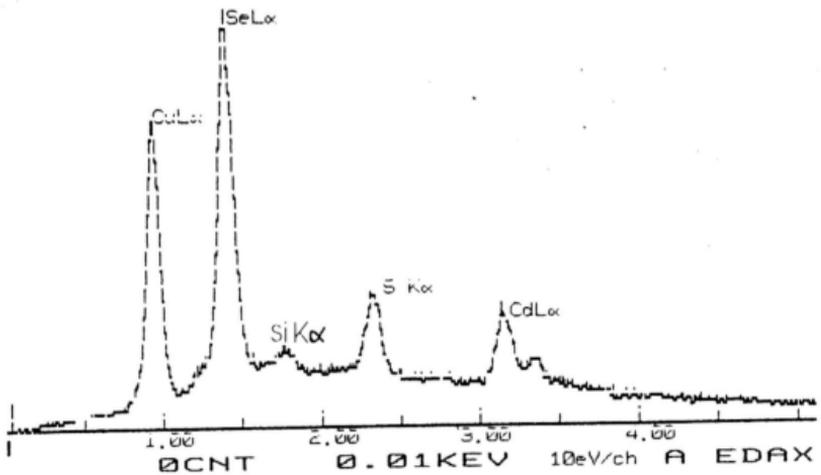
Figure 3.3b : EDX Spectra for CdSe Electrodeposited on Si at 0.7V for 120 minutes
