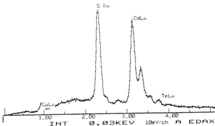
Figure 3.7c : EDX Spectra for CdTe Electrodeposited on Si at 0.8V
