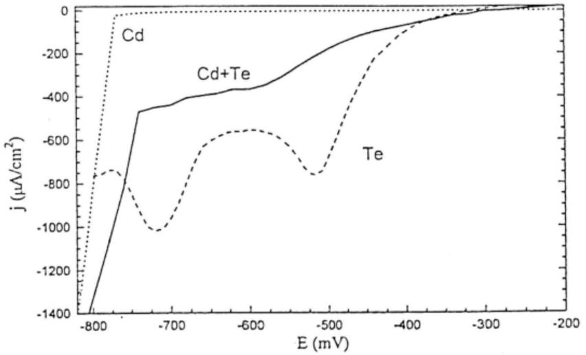
Figure 3.1 : Voltammogram for Cadmium (0.3M), Tellurium (1mM) and CdTe (Combined)
