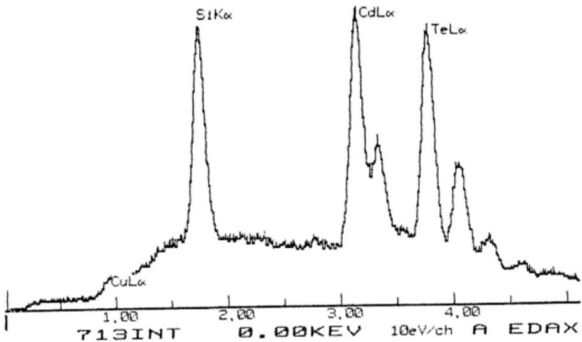
Figure 3.7b : EDX Spectra for CdTe Electrodeposited on Si at 0.67V
