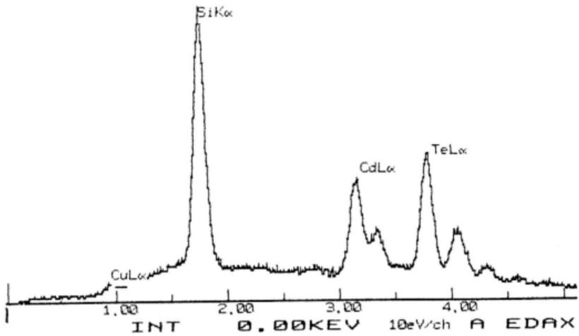
Figure 3.7a : EDX Spectra for CdTe Electrodeposited on Si at 0.45V
