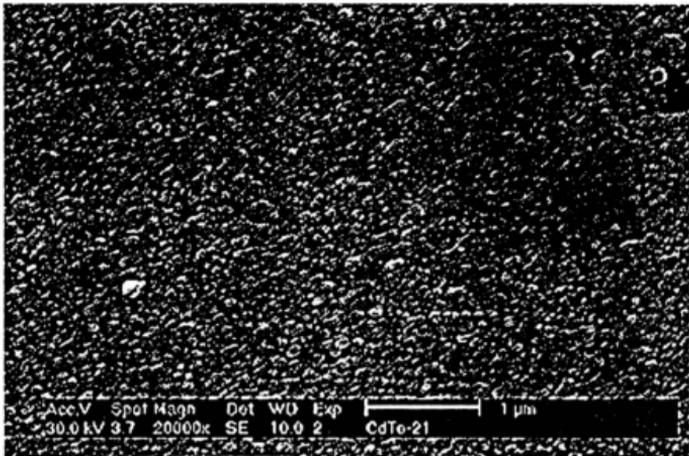
Figure 3.10c : Micrograph of CdTe Thin Film Electrodeposited on Silicon (20000X)
