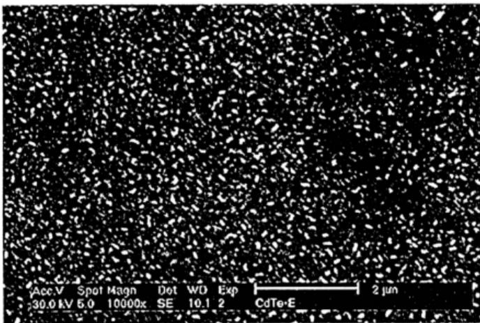
Figure 3.10b : Micrograph of CdTe Thin Film Electrodeposited on Silicon (10000X)
