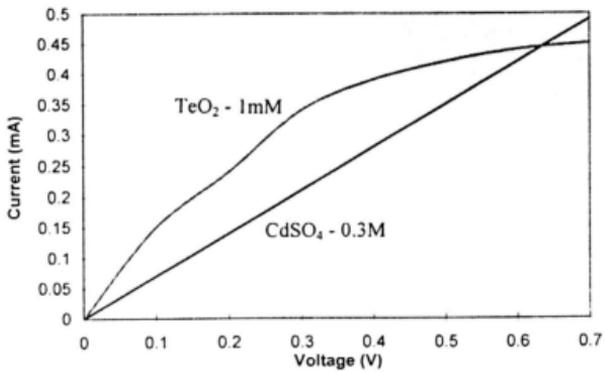
Figure 3.2 : Cathodic Polarisation Curve for Cadmium (0.3M) and Tellurium (1mM)
