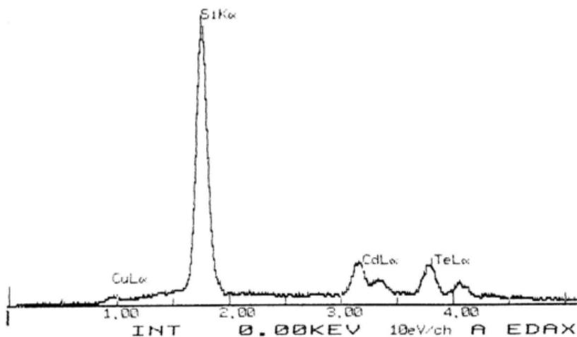
Figure 3.8a : EDX Spectra for CdTe Electrodeposited on Si for 10 minutes (at 0.67V)
