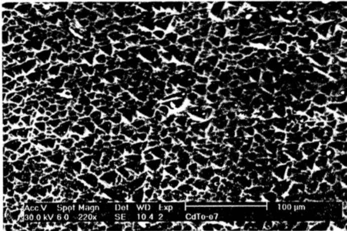
Figure 3.10a : Micrograph of CdTe Thin Film Electrodeposited on Silicon (220X)
