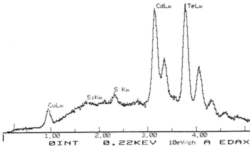
Figure 3.8c : EDX Spectra for CdTe Electrodeposited on Si for 60 minutes (at 0.67V)
