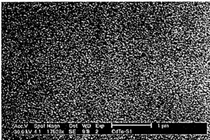
Figure 3.9b : Micrograph of CdTe Thin Film Sputtered on Silicon (17531X)
