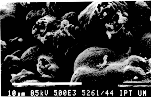
Plate 8B : Rupture in the gel film - evidence of budding after 72 h incubation at 30^{\circ} \pm 2^{\circ}\text{C} and 4 klux (whole bead)
