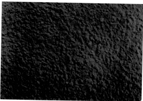
Figure 4.1.a : Light microscopic image of Si-Ti (paint II) panels after annealing at 863 K [ 590 °C] with the magnification 30X
