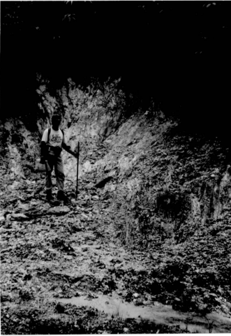
Plate 3.7 Light grey to whittish, highly weathered metaquartzite found exposed along the railway line (Location : ST 7 11km from Mambau)
