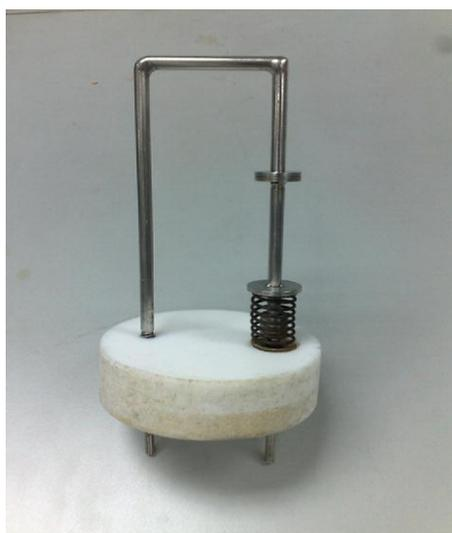
Figure 3.2: Conductivity holder with blocking stainless steel electrodes.
