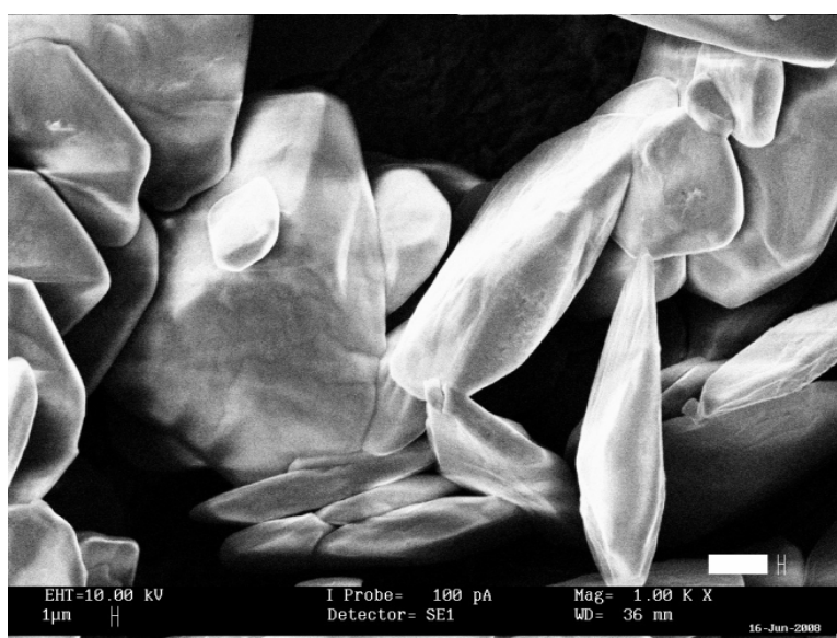
Figure 6.9: SEM surface morphology of 40[C4P6]-60AN film.
