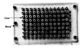
Figure 2.3: Pins on the block with gears pointing upwards
