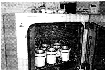
Figure 13. DHS Sampling Container and Oven System
