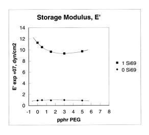
Figure 31: Storage modulus, E' versus pphr PEG for 0 and 1 pphr Si-69
