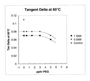
Figure 30 : Tangent delta versus pphr PEG for 0 and 1 pphr Si-69
