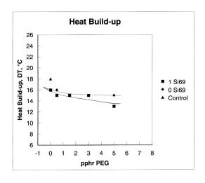
Figure 29: Heat build-up versus pphr PEG for 0 and 1 pphr Si-69
