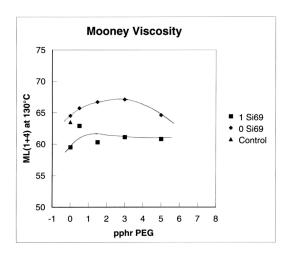
Figure 21: Mooney viscosity versus pphr PEG for 0 and 1 pphr Si-69
