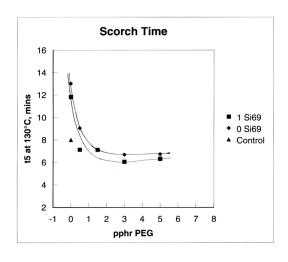
Figure 19: Scorch time versus pphr PEG for 0 and 1 pphr Si-69
