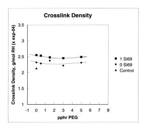
Figure 22: Crosslink density versus pphr PEG for 0 and 1 pphr Si-69
