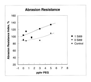
Figure 32 : Abrasion resistance index versus pphr PEG for 0 and 1 pphr Si-69
