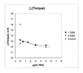
Figure 23 : Δ(Torque) versus pphr PEG for 0 and 1 pphr Si-69
