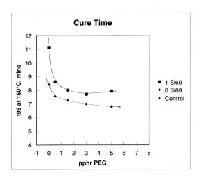
Figure 18: Cure time versus pphr PEG for 0 and 1 pphr Si-69
