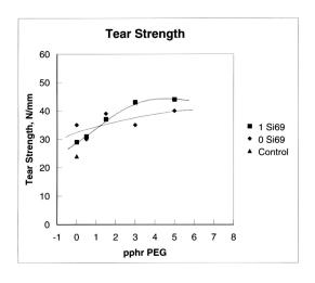
Figure 28: Tear strength versus pphr PEG for 0 and 1 pphr Si-69
