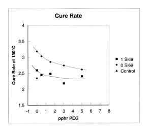
Figure 20: Cure rate versus pphr PEG for 0 and 1 pphr Si-69
