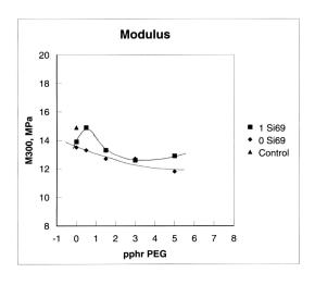
Figure 25: M300 versus pphr PEG for 0 and 1 pphr Si-69
