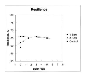
Figure 27: Resilience versus pphr PEG for 0 and 1 pphr Si-69
