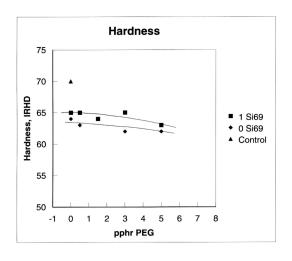
Figure 26: Hardness versus pphr PEG for 0 and 1 pphr Si-69
