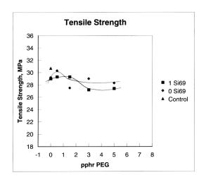
Figure 24: Tensile strength versus pphr PEG for 0 and 1 pphr Si-69
