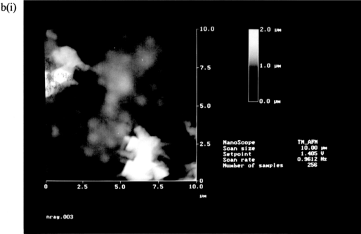
Fig. 2.14(b) Atomic force microscope images of WNR tube immobilised with HBsAg (i) 10x10 \mu\text{m} top view surface (ii) 10x10 \mu\text{m} three dimension surface 200 \mu\text{l} of HBsAg coating solution (1.76 \mu\text{g}/\text{ml} ) was incubated overnight at 4°C in WNR tube, (NR coated tube prewashed five times with 1 ml of 0.1M HCl followed by five washes with 1 ml of distilled water), the supernatant was then discarded and the tube was washed four times with 1 ml of distilled water.
