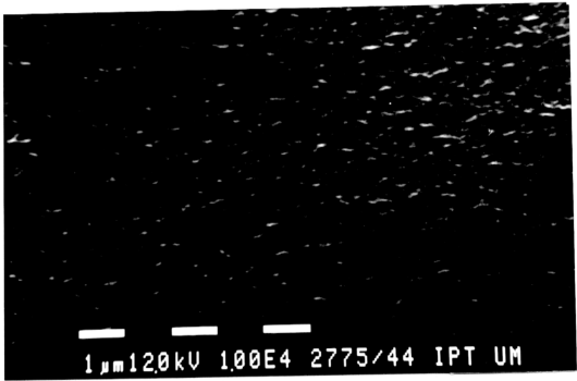
Fig. 3.10 (a) Scanning electron micrograph showing WNR surface. Magnification (i) 1 \times 10^4 WNR = NR coated tube was washed five times with 0.1 M 1 ml of HCl and followed by five washes with 1 ml of distilled water.
