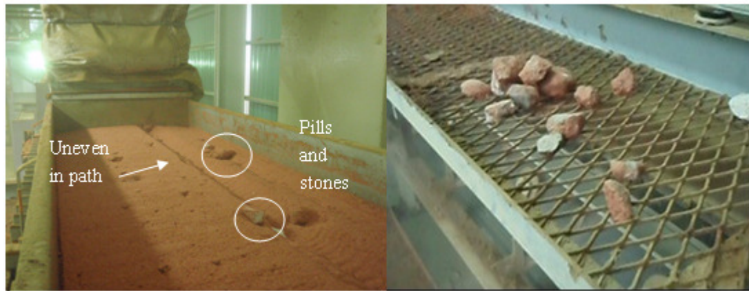
Figure 3.22 Pills and stones mixed in the raw materials create uneven weight distribution
