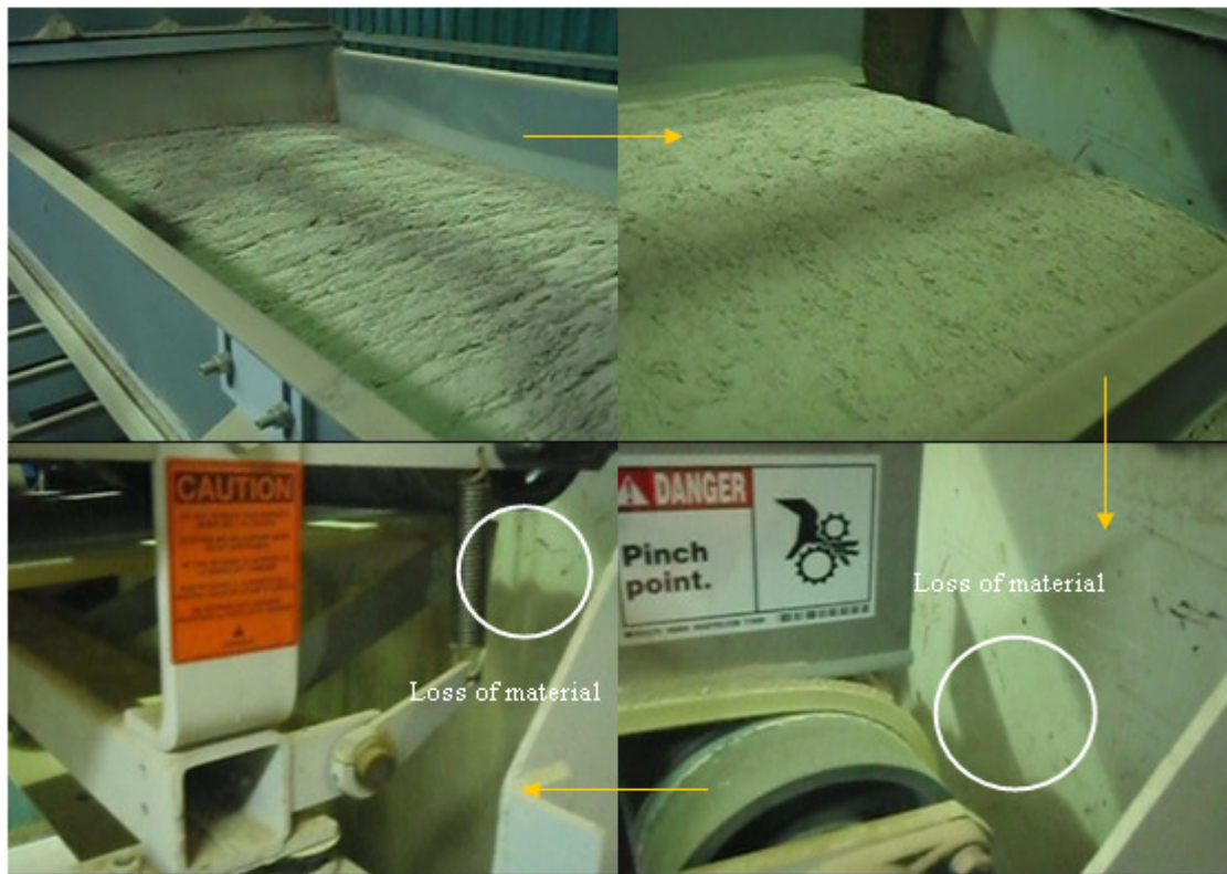
Figure 3.19 Loss of material occurs at raw material depot (stage 1)
