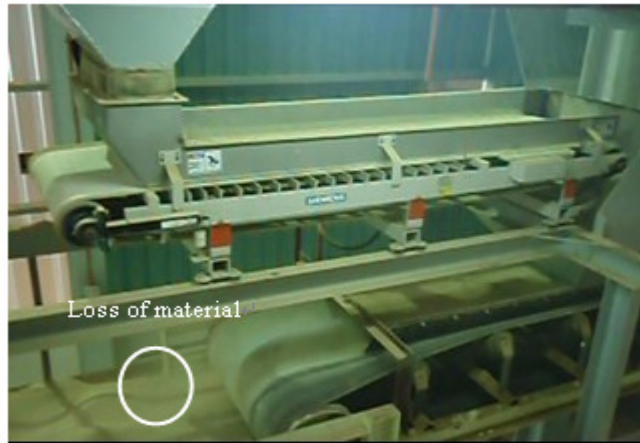
Figure 3.20 Loss of material occurs at stage 2
