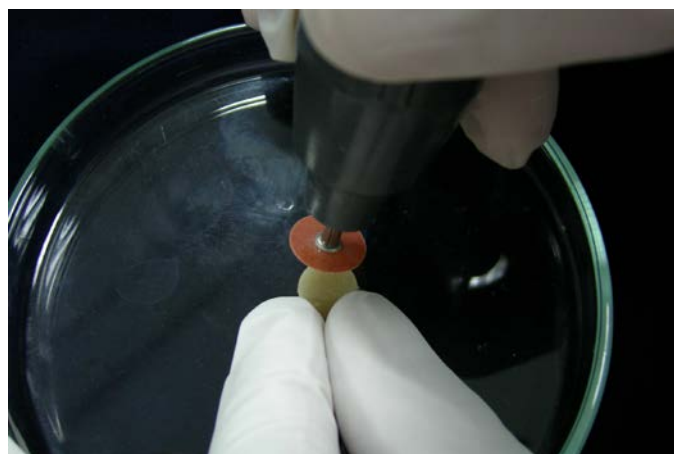
Figure 3.6 Polishing the specimen using soflex polishing disc with slow speed handpiece
