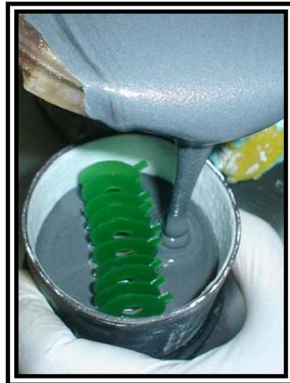
**Fig. 3.6.** The sprued discs invested.
