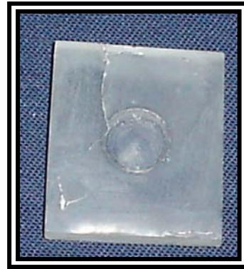
**Fig. 3.28.** The standardized cavity-epoxy-mould.
