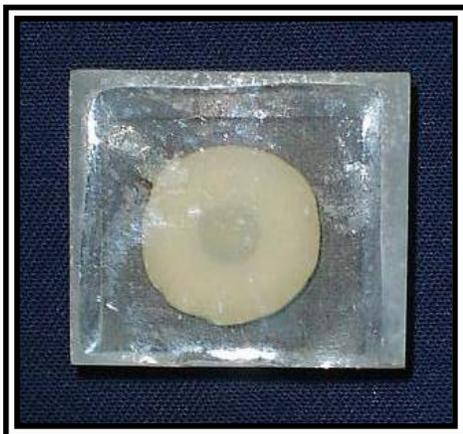
**Fig. 3.55.** Sample was embedded in epoxy resin.
