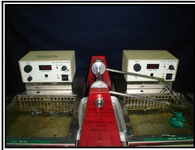
**Fig. 3.52.** The thermocycling machine used in this study.
