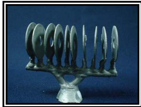
Fig. 3.8. The Casting was sandblasted.
