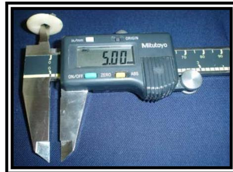
**Fig. 3.20.** Diameter of access opening.
