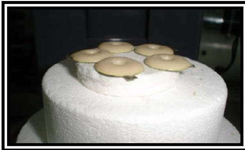
**Fig. 3.15.** The firing of body porcelain layer.
