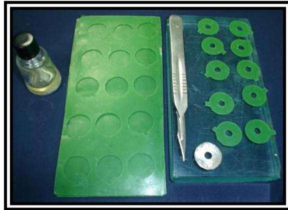
**Fig. 3.2.** Fabrication of wax discs patterns.
