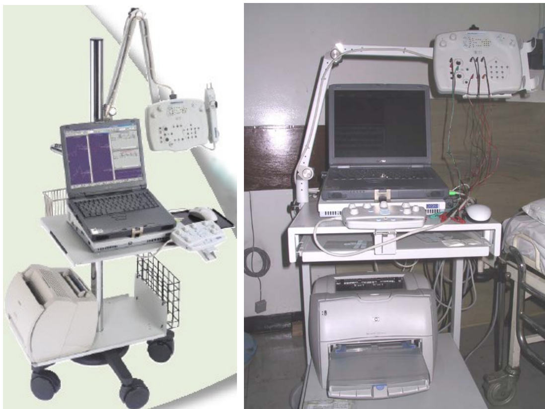
Figure 3.3.1(a) Five-channel system EMG equipment (Medelec Synergy N series, Oxford Instruments Medical, surrey, U.K.).
