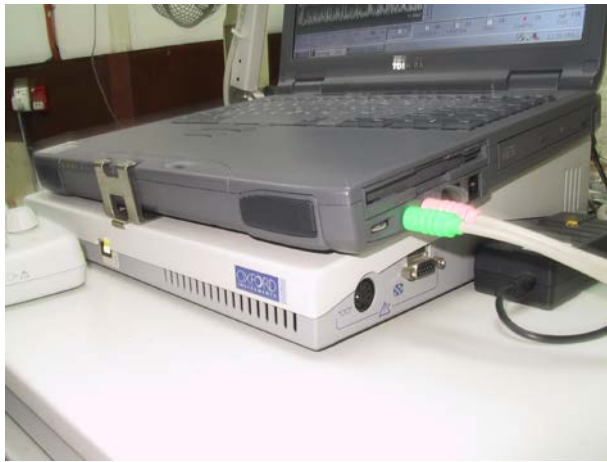
Figure 3.3.1(e) The plinth under the notebook is a central data acquisition unit that links together the computer, amplifier and control panel.
