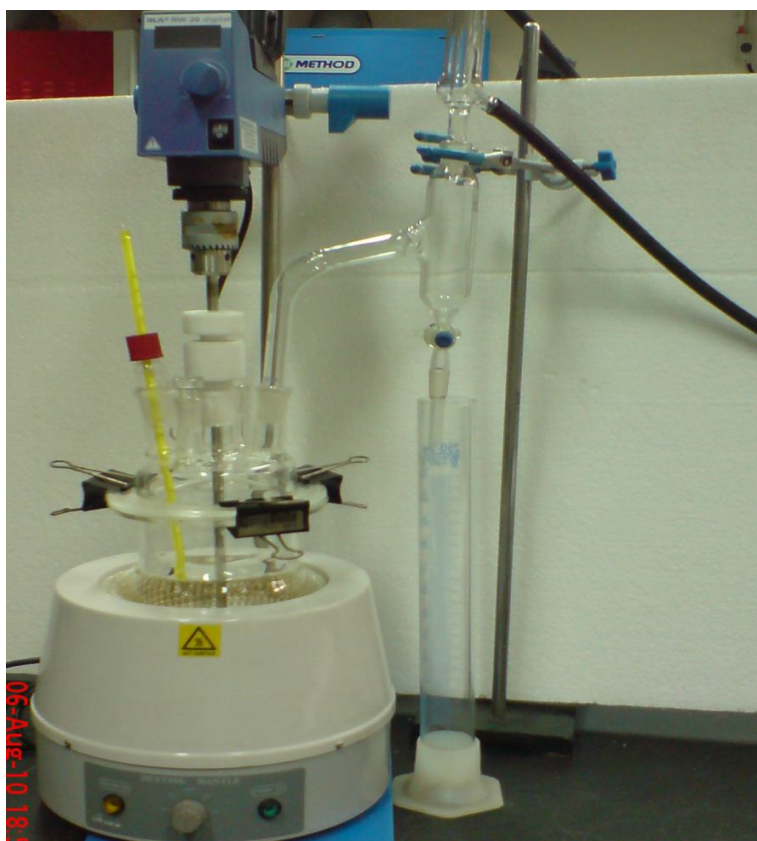
Figure 2.1 : Representation of set up used in polyesterification of macromers including reaction flask; Dean-Stark decanter; Condenser; Stirrer motor; Stainless steel rode of stirrer and Thermometer.
