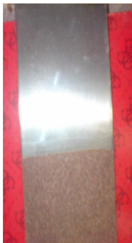
Figure 5.3 : Coated panel of AS3B(5%) sample after 8 months exposure in the open lab. bench (under hot and humid conditions)
