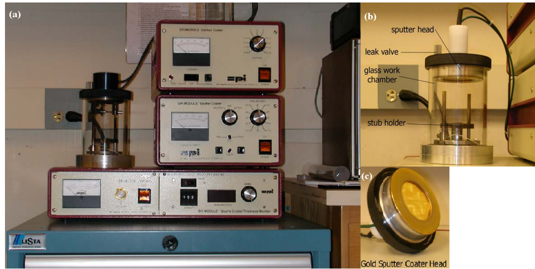
Figure 3.5. Sputtering system (model SPI) that was used in our lab for producing a gold coating on Si wafers.
