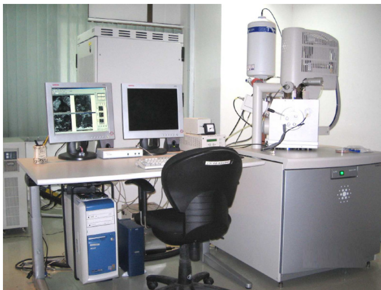
Figure 3.13. A photograph of the FEI Quanta 200F FESEM with EDX set-up.
