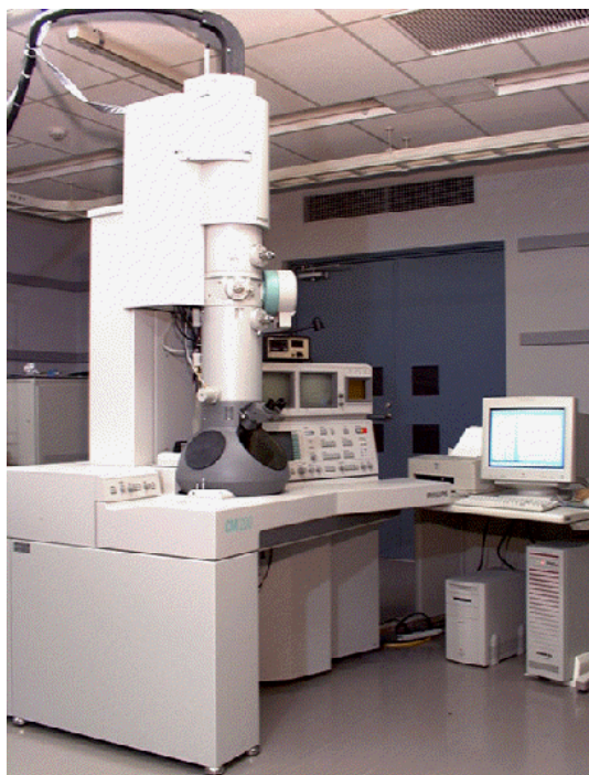
Figure.3.14 A photograph of the TEM microscope unit (Philips CM200).
