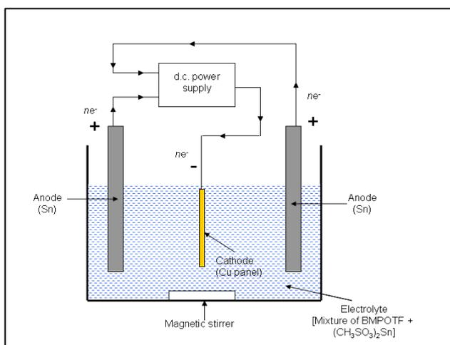
**Figure 3.22:** Schematic for an electroplating experiments
