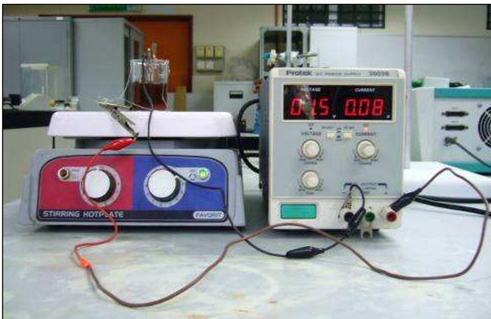
**Figure 3.21:** Electroplating experiments set up
