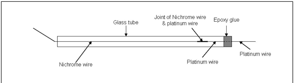
**Figure 3.19:** Structure of counter electrode- Platinum wire
