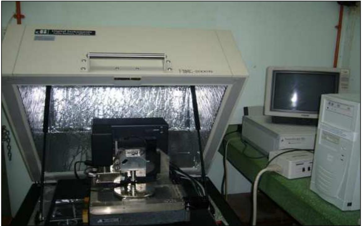
**Figure 3.7:** AFM: Digital Instruments Nano Scope 3a
