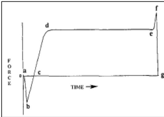
**Figure 3.14:** Typical wetting balance curve
