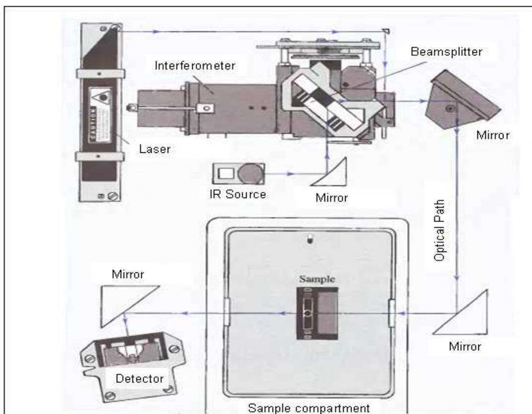
**Figure 3.10:** Instrument diagram for a basic FTIR spectrometer.
