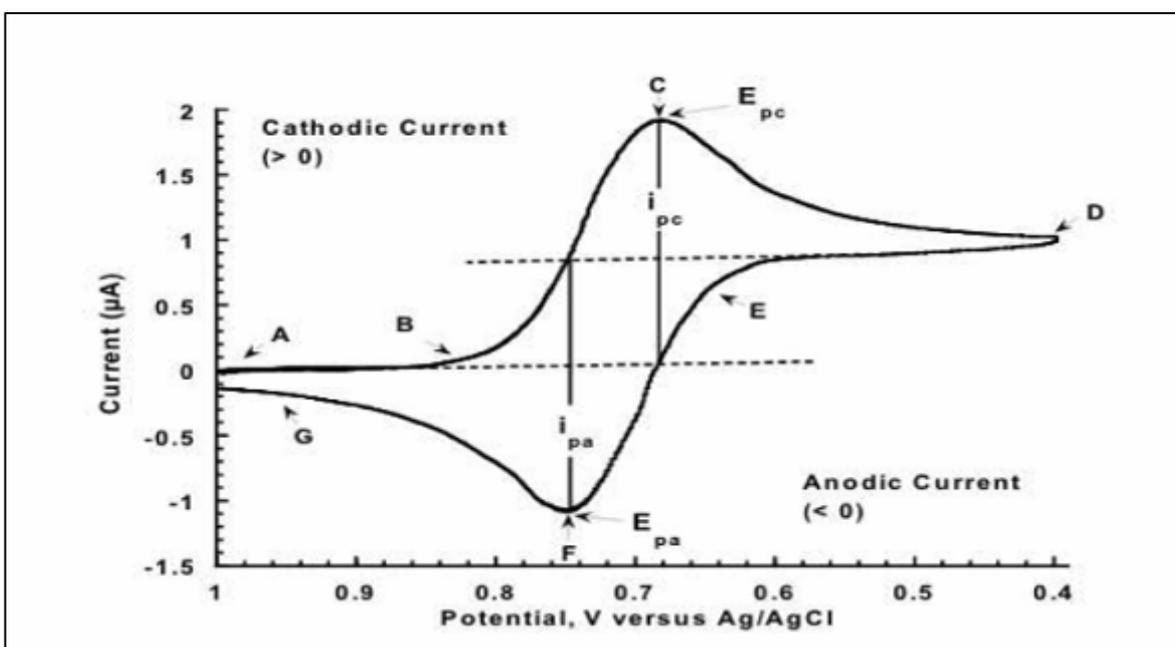
**Figure 3.2:** A typical cyclic voltammogram
