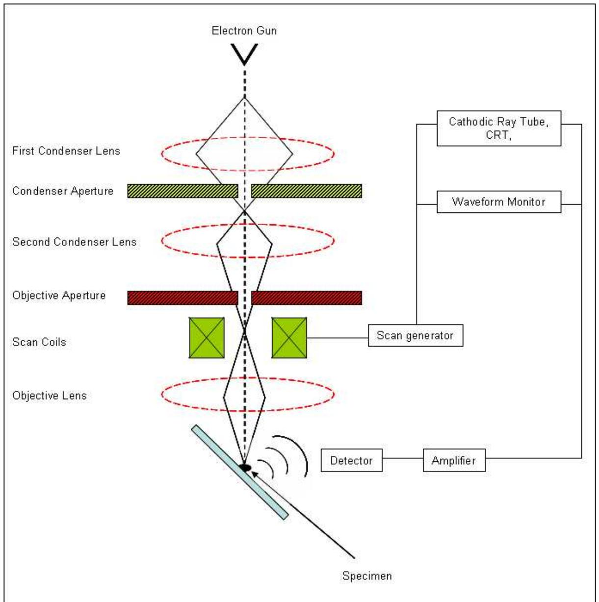
**Figure 3.5:** Schematic for an SEM
