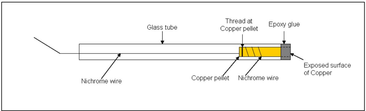
**Figure 3.18:** Structure of working electrode- Copper
