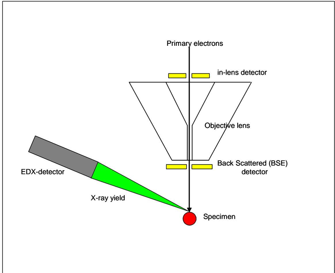
**Figure 3.6:** Schematic for an EDX
