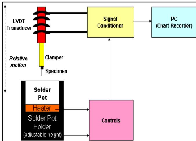
**Figure 3.12:** Schematic of wetting balance gauge
