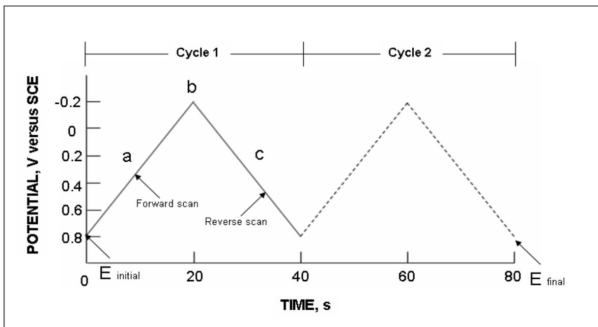
**Figure 3.1:** Typical excitation signal for cyclic voltammetry – a triangular potential waveform with switching potential at 0.8 and -0.2 V versus SCE
