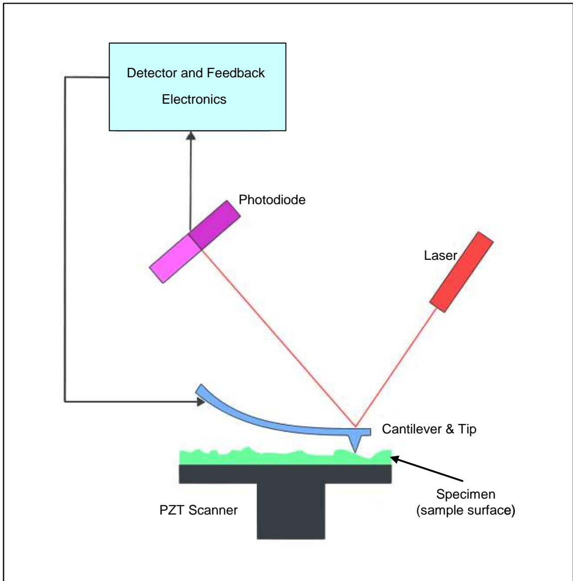
**Figure 3.8:** Schematic for an AFM
