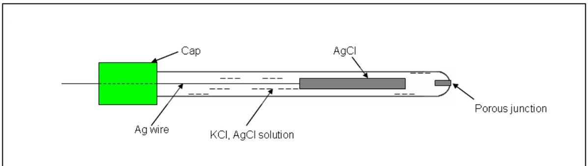
**Figure 3.20:** Structure of Silver-silver chloride reference electrode
