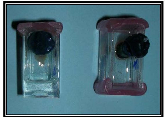
Figure 3.20: Specimen mounted in epoxy resin
