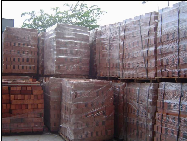
Figure 4.6: Storage of brick (Store in original packaging at open space until required)
