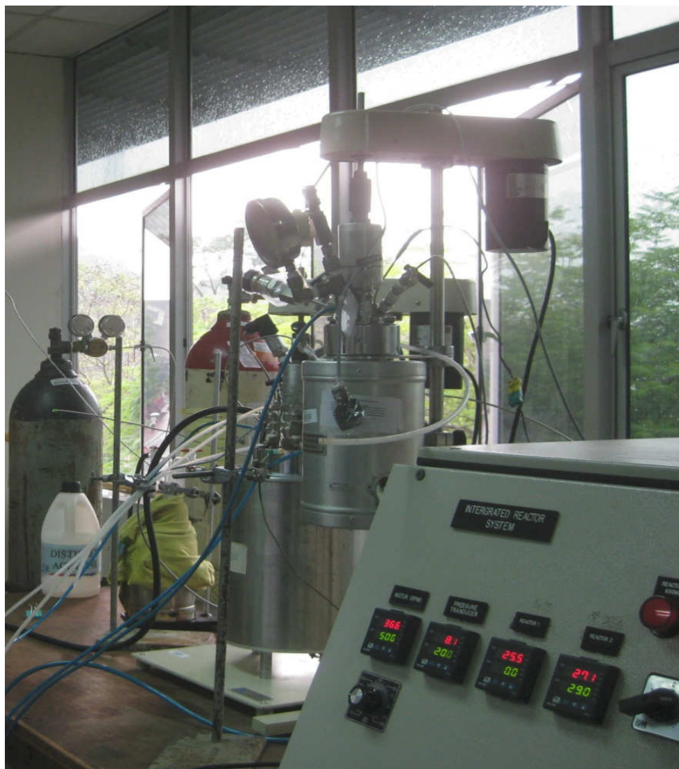
Figure 3.1: Layout of Parr Reactor
