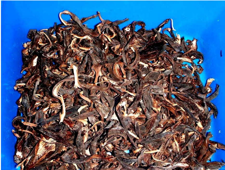
Plate 3.1 Dry banana skin used for bioremediation
