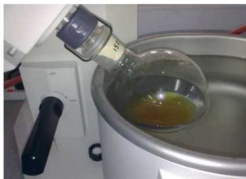
Picture 3.11 Solvents were distilled under reduced pressure at 40 °C in the rotary evaporator.
