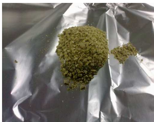
Picture 3.6 Dried rhizomes after being ground in the miller, ready to soak in the solvent.
