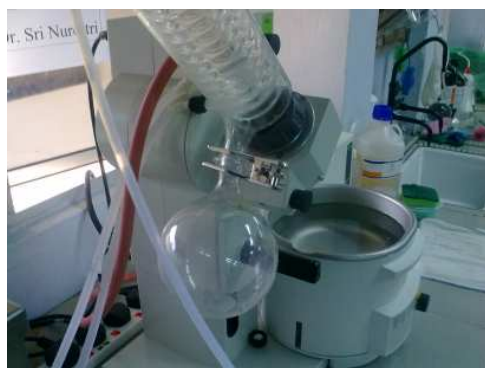
Picture 3.10 Rotary evaporator used to distill the solvents.
