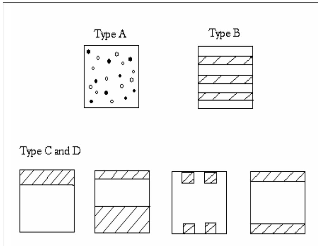
**Figure 1.1:** Schematic diagrams of hybrid types-all end view
