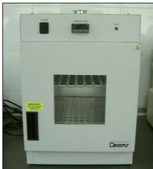
Figure 2.7: Oven to preheat the model for light-polymerized polymer
