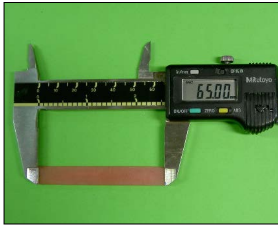
Figure 2.12: Length of specimen measured by micrometer
