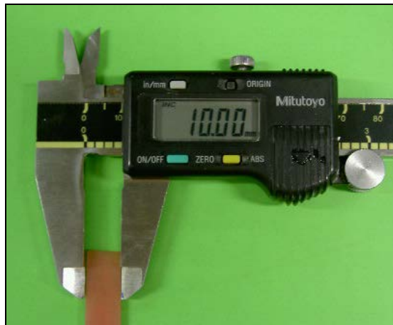
Figure 2.13: Width of specimen measured by micrometer
