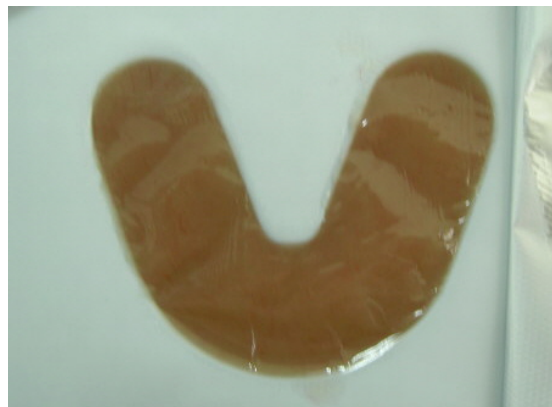
Figure 2.2: Light-polymerized urethane dimethacrylate denture base polymer material supplied in arch form
