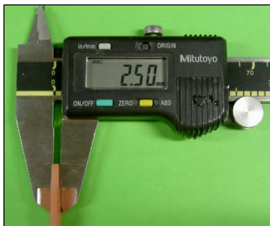
Figure 2.14: Thickness of specimen measured by micrometer
