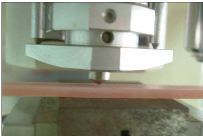
Figure 2.16: Close-up view of Shimadzu microhardness tester during the indentation of pyramid diamond indenter on the specimen
