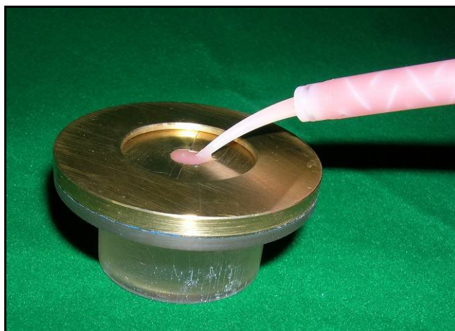
Fig. 3.21. Reline material being applied onto the denture base surface, which was confined in the brass ring.
