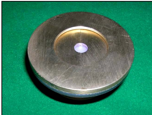
Fig. 3.20. Brass ring position on the mounted denture base specimen, with the denture base surface exposed in the centre of the ring.
