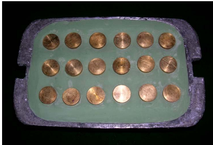
Fig. 3.7. Investments of brass columns in metal flask for Meliodent denture base specimens preparation.
