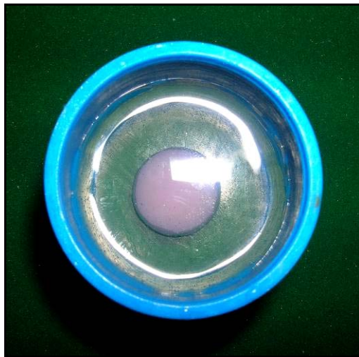
Fig. 3.14. Denture base specimen embedded within epoxy resin in the mounting cup.
