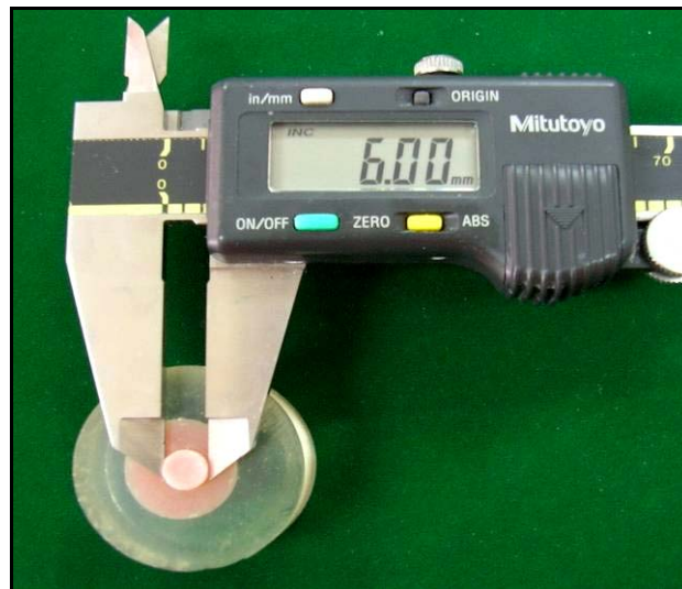
Fig. 3.23. The diameter of specimen being measured using a digital micrometer (Mitutoyo Mfg.)
