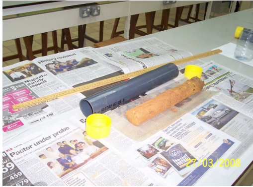
(b) Soil sample was taken out from the plastic cylinder
