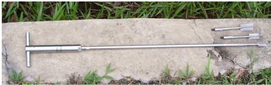
Figure 3.3 A vane tester (Eijkelkamp Agrisearch Equipment model 14.05, The Netherlands) used to measure soil shear strength.
