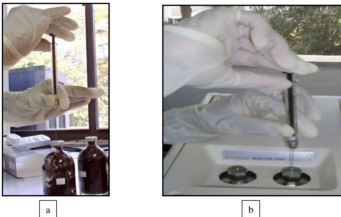
Plate 3.4: (a) Injecting out gas sample from Wheaton bottle
