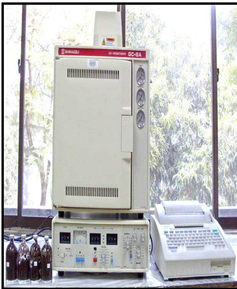
Plate 3.3: The Gas Chromatography model Shimadzu 8A used for the analysis.
