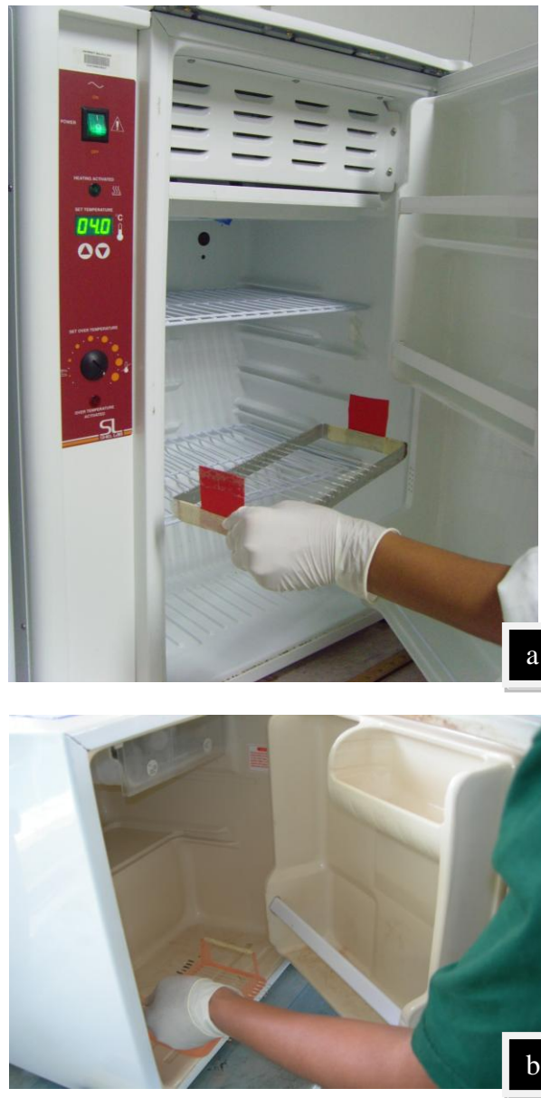
Figure 3.8: Equilibration phase. (a) Equilibrated using low temperature incubator under laboratory ambient; (b) Equilibrated using normal refrigerator under field condition.
