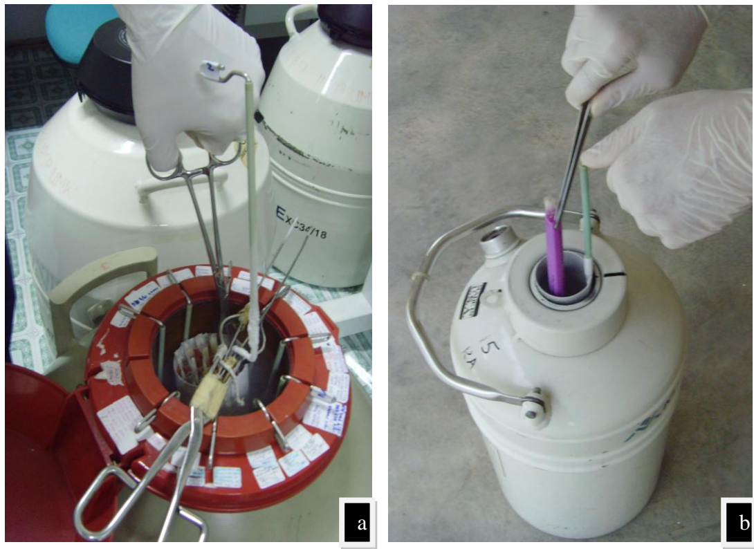
Figure 3.10: Storage of frozen sperm in LN 2 tank. (a) Storage in LN 2 storage tank under laboratory ambient; (b) Temporary storage in LN 2 carrier tank of frozen sperm after undergo freezing process under field condition.
