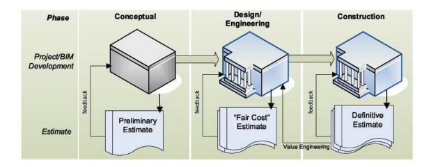
Figure 6.1: Project phases and cost estimating method (abstracted from: Sabol, 2008)
