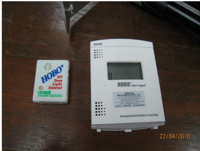
Figure 5.5(a): HOBO data logger to measure air temperature, relative humidity and daylighting
